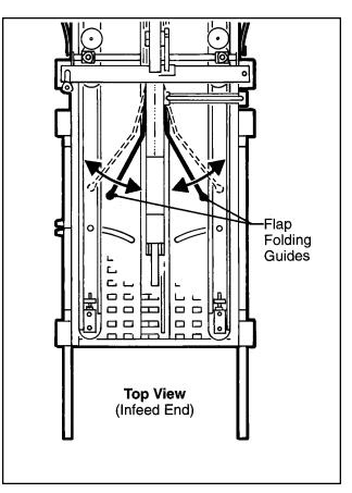
Figure 3-12 – Box Size Set-Up
